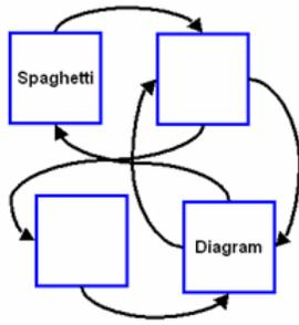
Spaghetti Diagramming also uses Post-it notes, but this time to diagram a workspace and show how the product or service, people and materials move around in it. Again, an hour or two analyzing the movement of people and materials in the workspace will identify ways to reduce unnecessary movement by 50% or more. This will also reduce mistakes and errors. It's harder to misplace something when it doesn't have to move too far.
