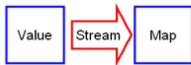
Value Stream Mapping (VSM) uses Post-it® Notes to show the process flow. I use square Post-its for actions and arrow-shaped Post-its for the gaps between actions. A small team of people can usually diagram the current workflow in an hour or less. When we start putting times on each of the actions and arrows, members quickly find that most of the delay is in the arrows. Often, one or two arrows consume most of the total delay.
